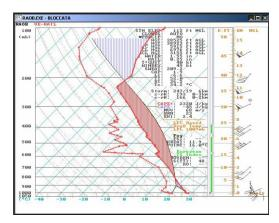
The SkewT image at left is a sample of the RAOB 4.0 program. The 4.0 program was the last version created for the MS-DOS environment. It also had capability to create Hodographs and Cross-Sections, and even had a Soaring display screen. Ever since its release in 1998, it is still in use around the world, and John continues to provide free technical support to its users.
